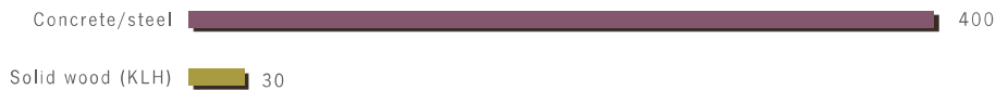
Illustration 18 – Comparison of CO 2 emissions between the constructions Source: Dem Klimawandel entgegen, www.cei-bois.org
